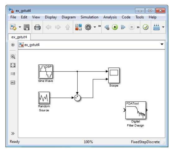
**2** Incorporate the Digital Filter Design block into your block diagram by placing it between the Random Source block and the Sum block.
